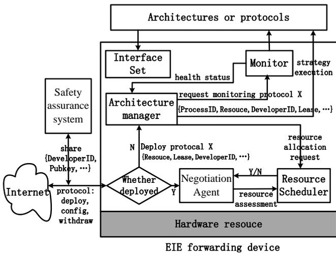
Figure 3. The whole EIE components interaction mechanism
