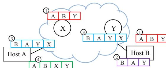
Figure 6. Host protocol stack supports AS landmark option in packet header. Packet format (B, A, Y, X) means source address is host B's IP address, destination is host A's IP address, source landmark is Y, and destination landmark is X; the numbers in circle mean the step sequence.
