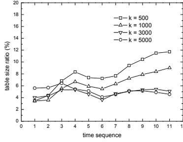
Figure 8. Select ASes of degree top  $k$ , and strict AS landmark routing
