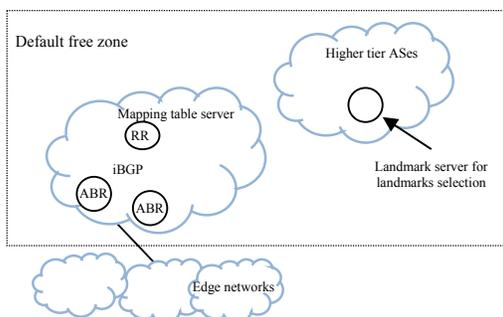
Figure 5. A centralized structure for landmark selection and mapping table creation.
