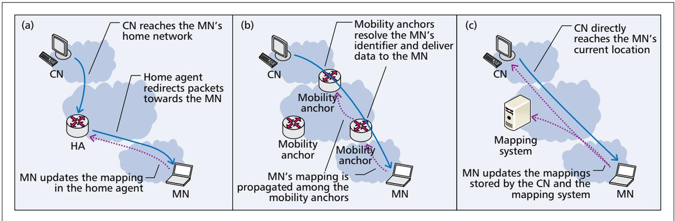
Figure 1. Illustration of a) Mobile IPv6; b) distributed mobility management solutions; c) ILS designs.
