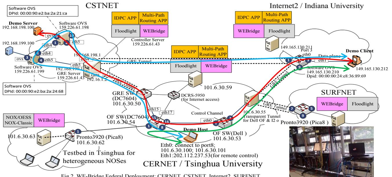
Fig. 2. WE-Bridge Federal Deployment: CERNET, CSTNET, Internet2, SURFNET
