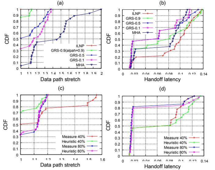
Figure 2. Cumulative Distributed Function (CDF) of data path stretch and handoff latency of (a, b): MHA, ILNP and GRS with different  $\alpha$  and  $\beta$  values; (c, d): direct measurement and distance prediction
