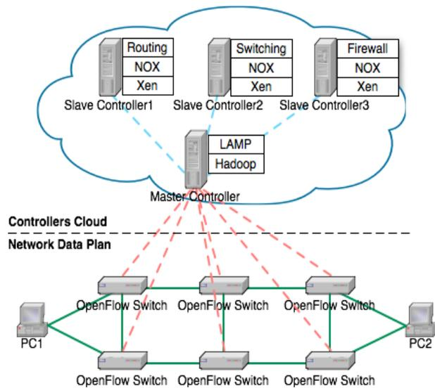
Figure 3. An initial prototype of Cloud-based network.
